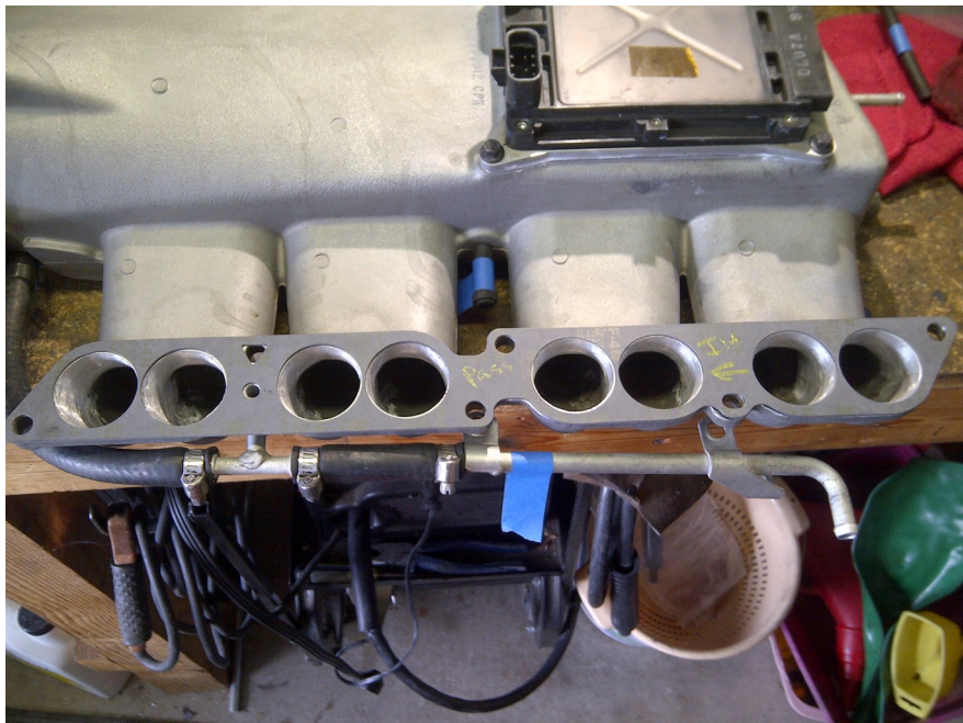
Intake manifold after grinding with gasket demonstrating the alignment and diameter increase of the port at the mating surface.
