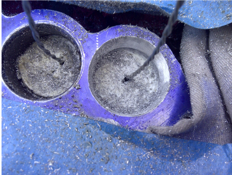
Injector housing port almost finished. Note the pitting on the edge probably caused by misalignment air flow turbulence.
