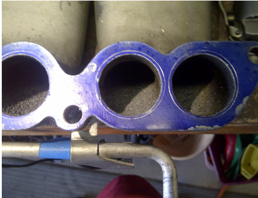
Scribe marks in the layout fluid. Note the radial misalignment.
