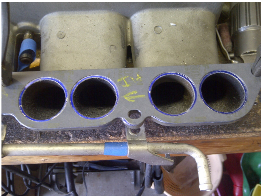
Mismatch of gasket and intake manifold ports.
